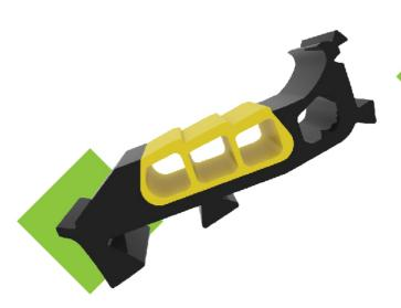
New Generation Integrated Seal for concrete pipe and manhole systems. Sealing part EPDM 40 IRHD, secondary part made of hard rubber 85 IRHD, reusable. Improved functionality at reduced cost
